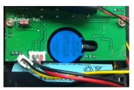
battery will only charge when the AW07A is off. For charging the position of the EXT PWR-BAT jumper does not matter. It will charge in either position. To switch between the AA cell pack and the rechargeable 18650 unplug the 3 pin header from the AA cell pack
