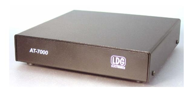
Your AT-7000 is powered directly by the radio; it needs no separate power supply. Your AT-7000 automatically powers up whenever you start a tuning cycle, and after tuning, automatically enters a "deep sleep" state in which it draws less than 8 mA. The tuner will automatically "wake up" the next time you start a tuning cycle. The latching relays hold the tuned configuration indefinitely, even while DC power is completely removed. Tuning memories are stored indefinitely in EEPROM memory.
